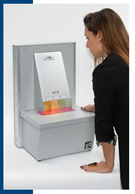
The Simultaneous Color Viewer (SCV) is a desktop viewer designed to show the effect different light sources will have on a single color or color pairing placed side-by-side. The SCV enables you to detect metamerism and test for color harmony.
